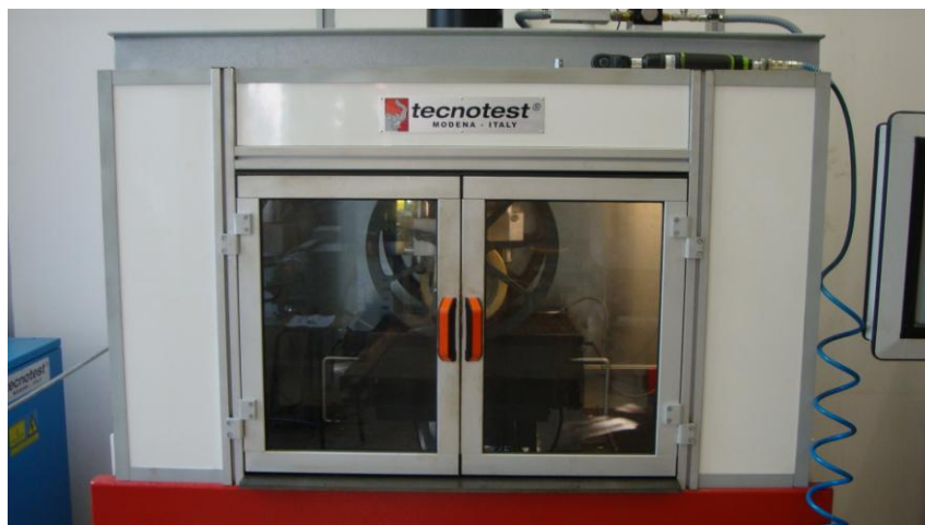
Figura 28 Wheel Tracking Test: prova in atto
