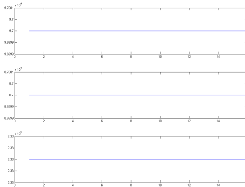
Figure 4.8: No matter which covariance matrices we choose, the estimates are not worsened if we make an exact guess. This is a plot of the values of \beta (in order: vessel 1, vessel 2 and vessel 3) against the estimation step.
