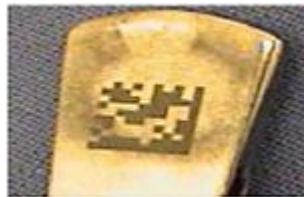
Figure 4.12 Example of laser engraved DATAMATRIX code [Tamagno, 2008]
