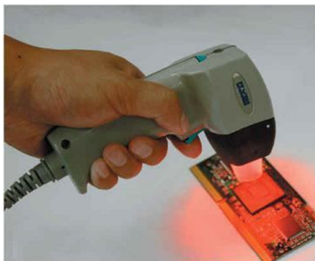
Figure 4.11 : DATAMATRIX reader scans and acquires a code applied on an electronic plate [hte.net]
