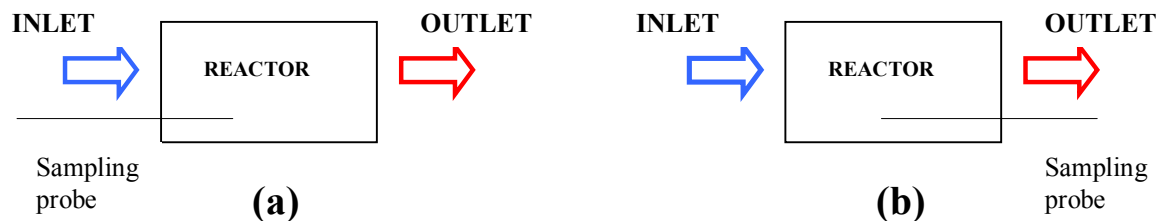
Figure 4.13: Sampling from the cold side of the reactor (a) and sampling from the hot side of the reactor (b).
