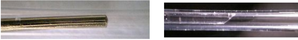
Figure 4.1: Fused silica capillary containing thermocouple (left) and optical fiber (right).
