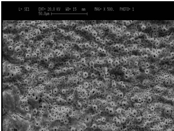
Fig. 3.28: SEM pictures of SUM AgNPs sample after flexion of 30°.
