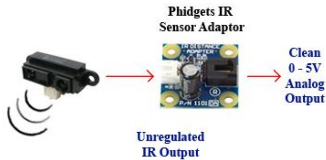
Figure 104 : GP2D12 Sensor interface with IR adaptor
