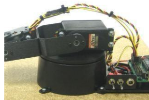
Figure 42 : Cable arrangement of the arm
