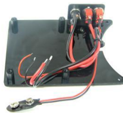
Figure 16 : Battery wire connection
