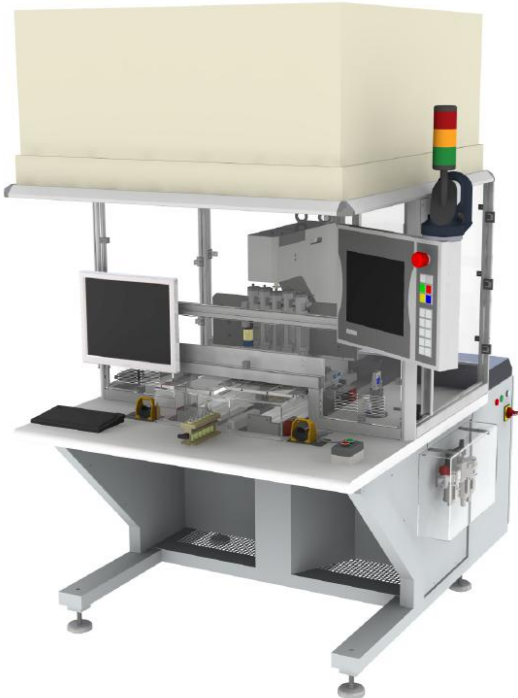
Figure 11 - Hakim Valve Semi-Automatic Assembly Machine
