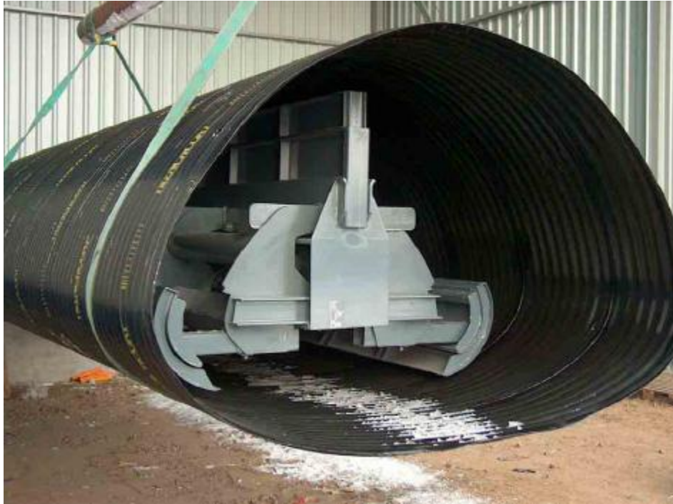
Figure 3.14 – Machine to define pipe arches
