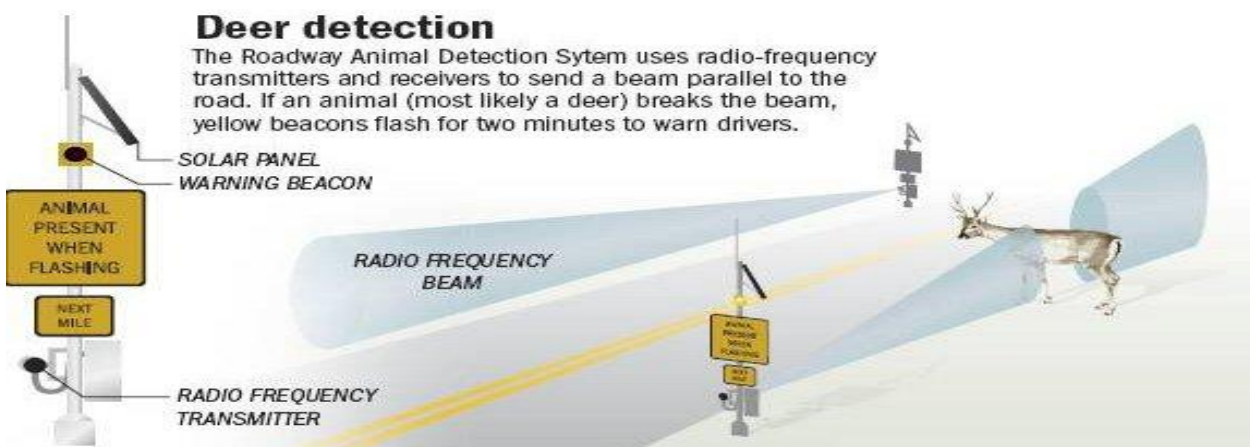
Figure 6.14: Animal detection systems
