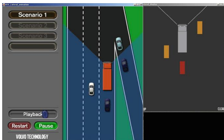
Figure 6.24 Lateral area monitoring and information presented to the driver in a truck
