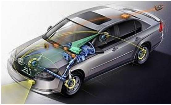
Figure 6.10: Active Front Steering
