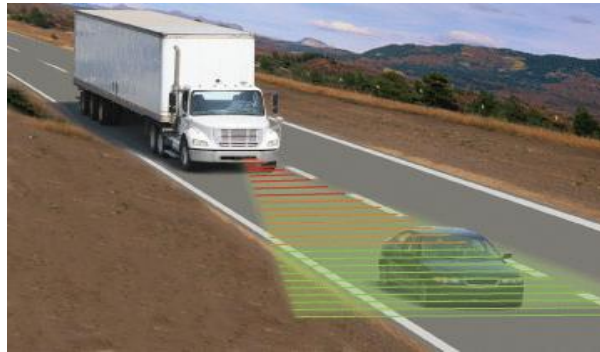
Figure 6.18: Forward distance warning
