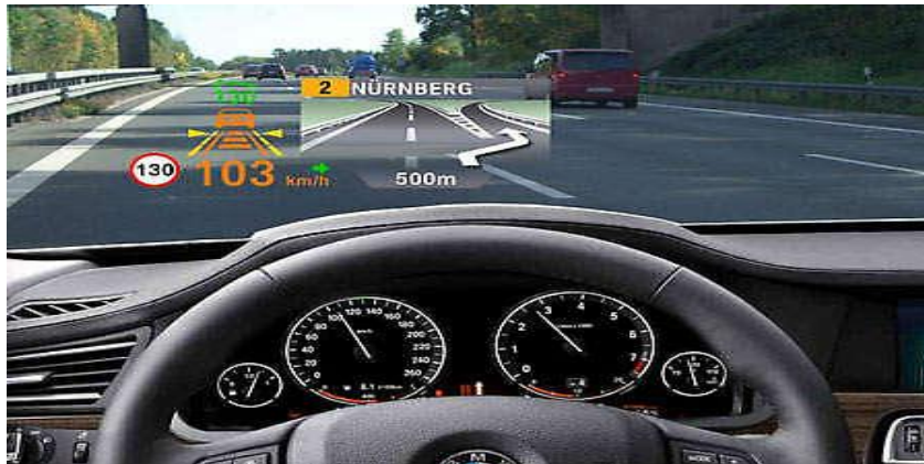
Figure 6.20: Head Up Display
