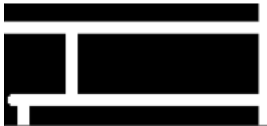
Figure 3.3: An example of map, where each pixel represents a cell of a predefined size.
