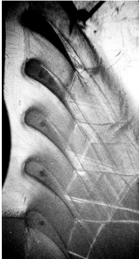
Figure 2.7: The shock wave coming out from the trailing edge of each blade, bouncing against the upper wall and reflected over the next blade (Schlieren picture [33])
