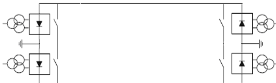
Figure 5.13: Bipole with Earth Return
