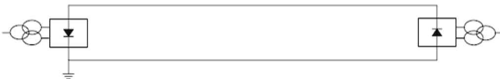
Figure 5.11: Monopole with Metallic Return
