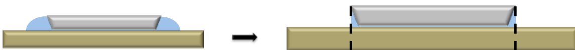
Figure III.17: the excess of adhesive in the first samples was cut perpendicularly to the edges.
