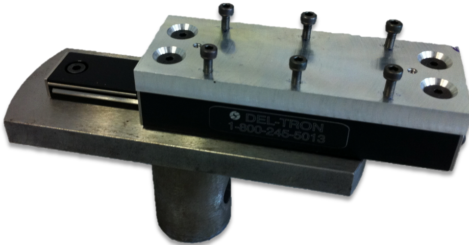
Figure III.12: trolley used for the peel tests; the screws hold the fixed arm in position.
