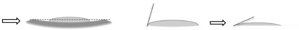
Figure III.6: the distortion of the substrate causes the camera to record a wrong contact angle.
