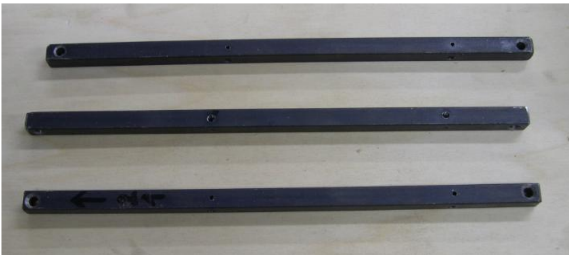
Figure 62 Steel rods used to keep the probes in position
