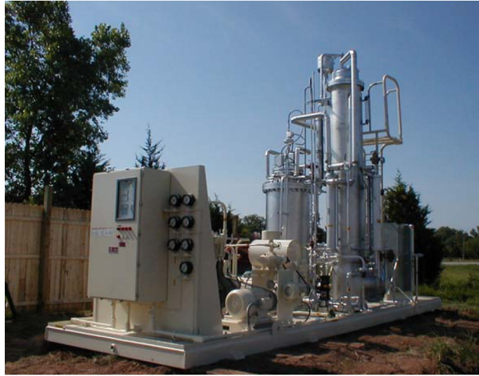
Figure 2.24: GTL mobile plant (source: Alchem)
