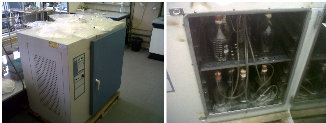
Figure 3.3: BMP tests in progress
