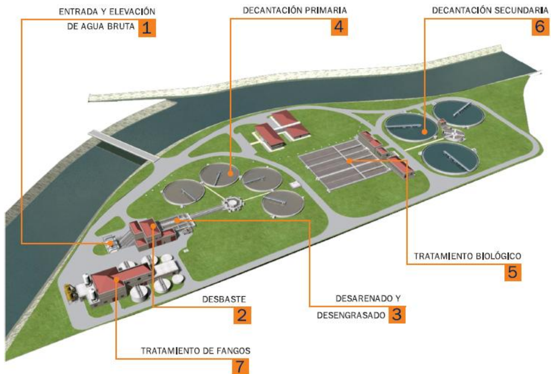
Figure B.1: Schematic of the Frieres wastewater plant, bordered by the Nalón river: (1) raw water inlet and lift, (2) grinding, (3) grit and grease removal, (4) primary sedimentation, (5) biological treatment, (6) secondary sedimentation, (7) sludge treatment
