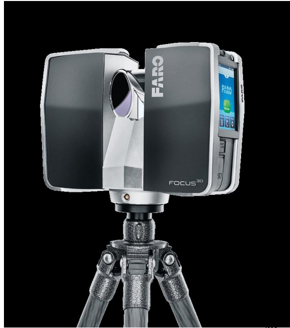
Figure 2.1 FARO Laser scanner Focus 3D
