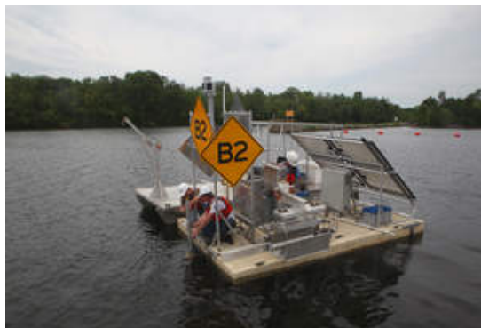
Figura 3.2.1, fonte Beacon Institute
