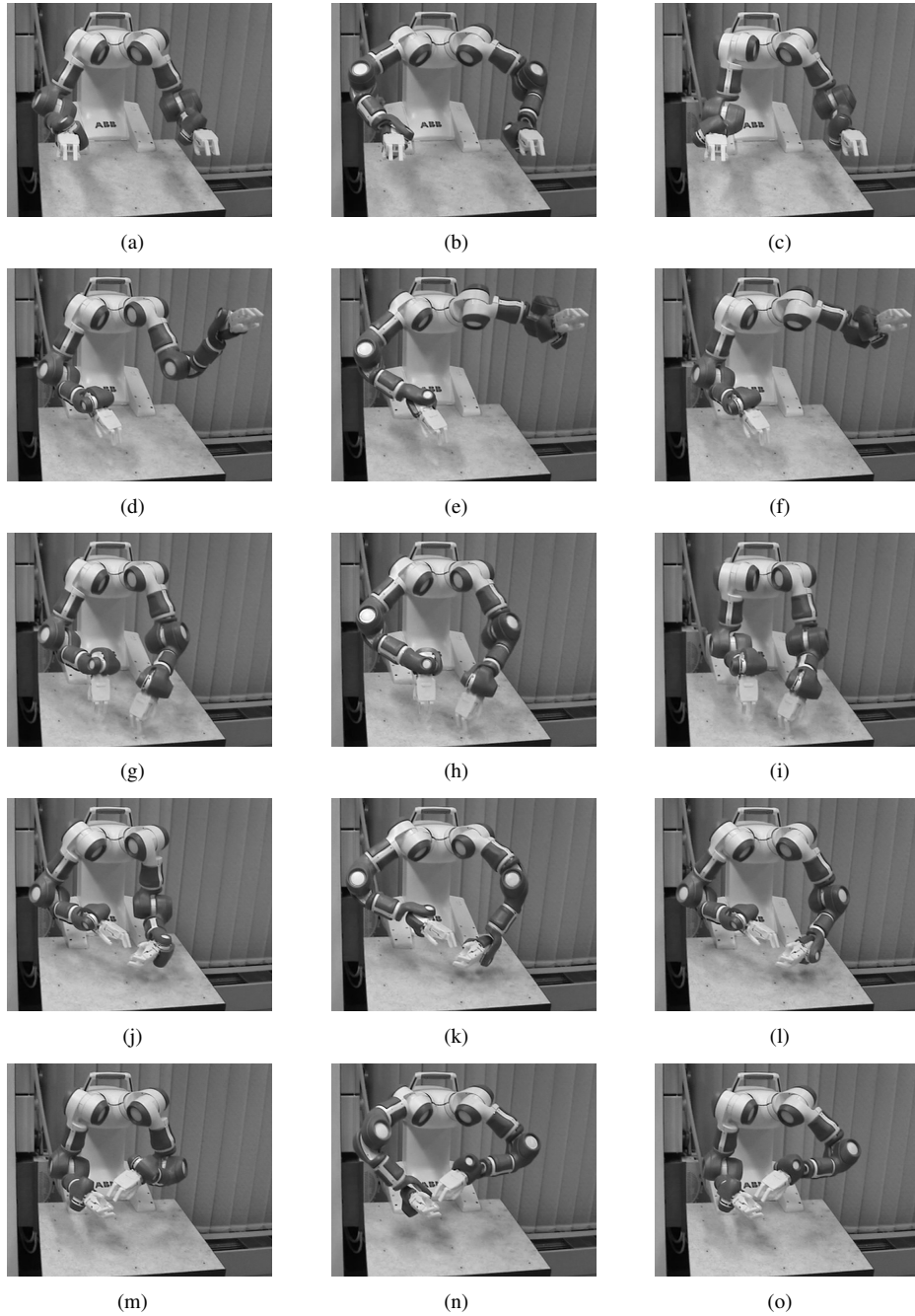
Figure 6.6: Three redundancy resolutions for the prototype robot (left: HL, center: nHL, right: GnC)
