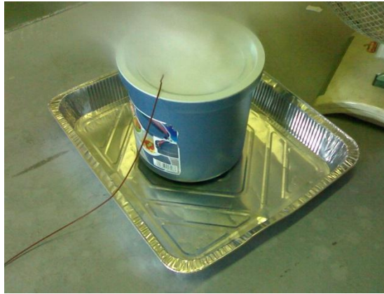
Figure 3.9. Ethanol-liquid nitrogen bath inside the thermal vessel
