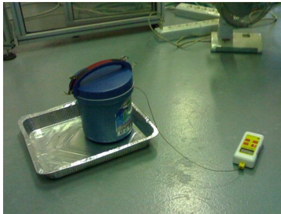
Figure 3.8. Image of the insulated vessel for Charpy specimens cooling whose temperature is controlled by a thermocouple
