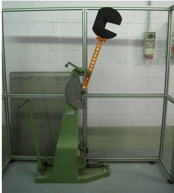
Figure 3.10. Charpy pendulum for Impact tests presents at Falco laboratories (Politecnico di Milano)
