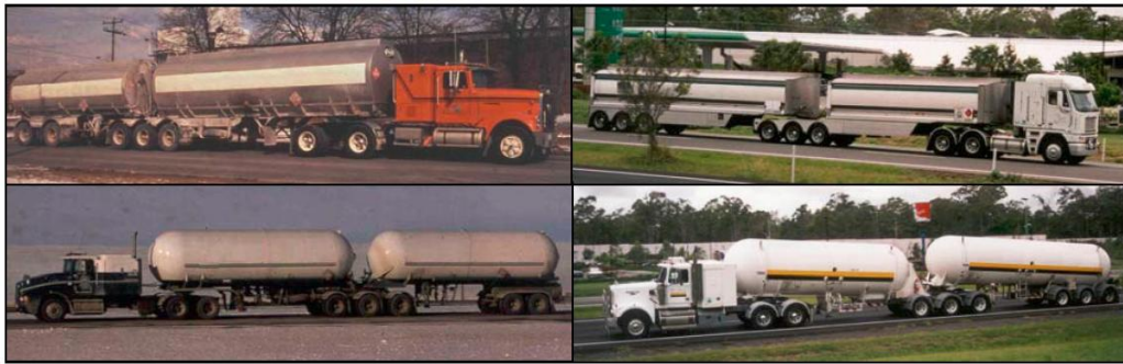
Figure 2.2: Comparison between Australian (right figures) and Canadian (left figures) B-train for carriage of liquid fuel (top figures) and liquid propane (bottom figures)
