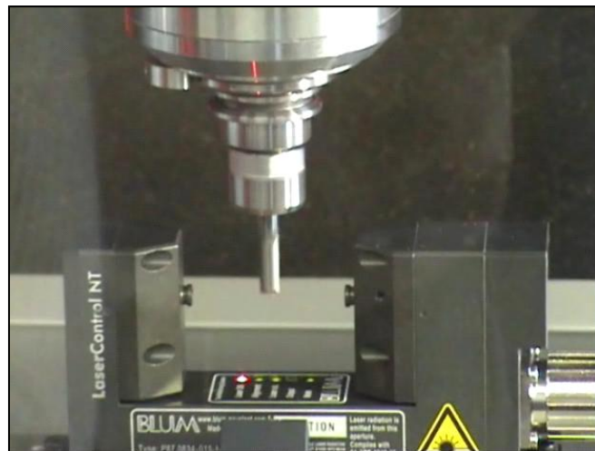
Figure 2.2. Laser presetting system during the measurement of a mill.
