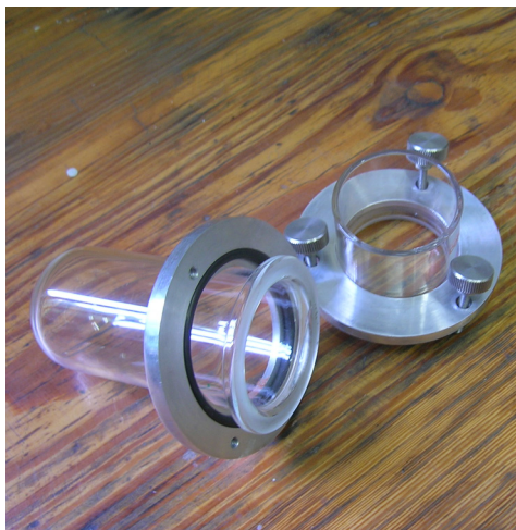
Figure 3 - Ad hoc test tube used for permeability characterizations.
