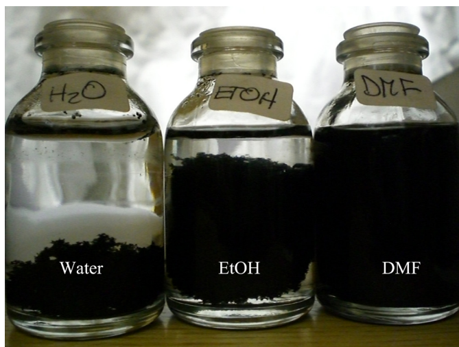
Figure 3 - Picture of the dispersions of CNT in different solvents, taken after 30 minutes of dispersion preparation.
