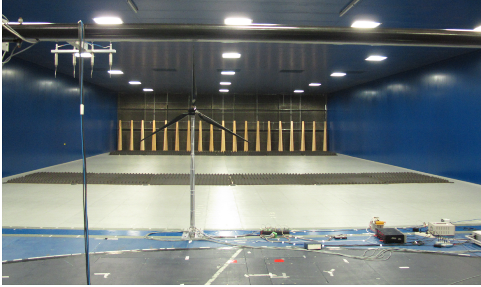
Figure 5.1: Image of the experimental setup for wind tunnel wake measurements on the wind turbine. It is possible to identify the spires, the floor roughness. Close up are visible the cobra probes used for the measurement of the velocity in the wake of the wind turbine.
