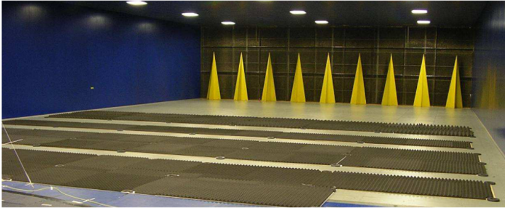
Figure 3.1: Wind Tunnel setup with spires and floor roughness.
