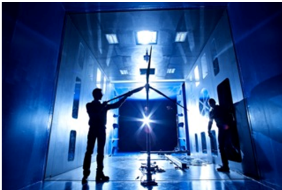
Figure 4.2: Wind turbine installation in the high-speed low-turbulence test section at Politecnico di Milano Wind Tunnel [3].
