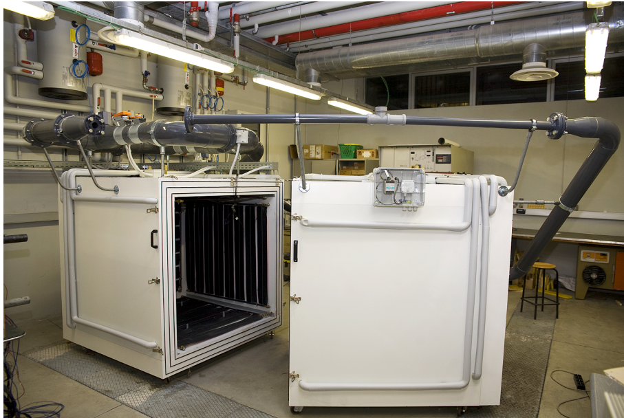
Figure 6.6: Picture of the overall apparatus at the end of the construction process. The measurement section is visible.
