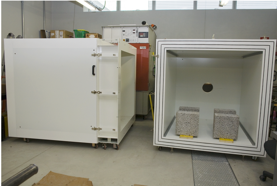
Figure 6.1: Picture of both chambers of the DAVTB apparatus as they have been produced by the manufacturer. In the right one the hole for the connection with the ventilation system is visible. The frame for the sample housing is visible too (in the picture is connected to the box on the left side).
