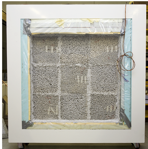
Figure 6.8: Wall sample made of no-fines concrete blocks. The edge insulation made of polystyrene slices is visible.
