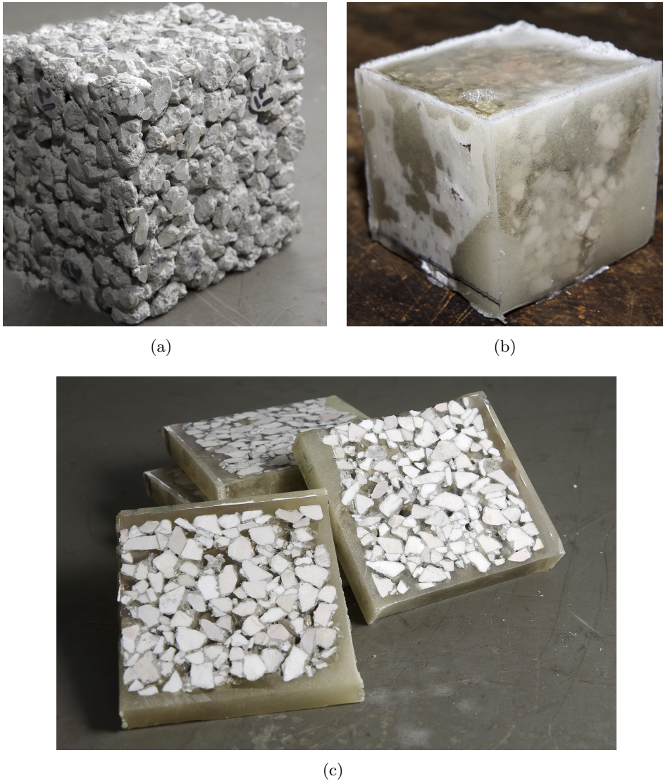
Figure 4.1: (a) Picture of a cubic sample of no-fines concrete (this particular one has not been used for experimental purposes, because of some inaccuracies in the casting procedure). (b) Picture of one sample impregnated in the hardened epoxy resin. (c) Picture of one impregnated sample cut into slices.
