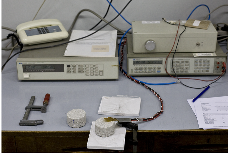
Figure 4.9: Picture of the TPS apparatus: on the right side there are the multimeter (bottom) and the Wheatstone bridge; on the left side there is the power supply. On the bottom of the picture there are the circular probe and one of the concrete samples used in the experimental analysis.
