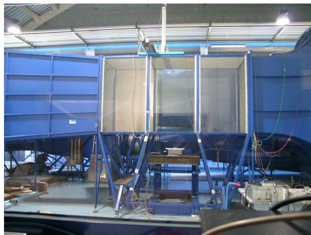
Figure 2.1: Test section of the low-speed wind tunnel at the Aerodynamics Laboratory of Politecnico di Milano
