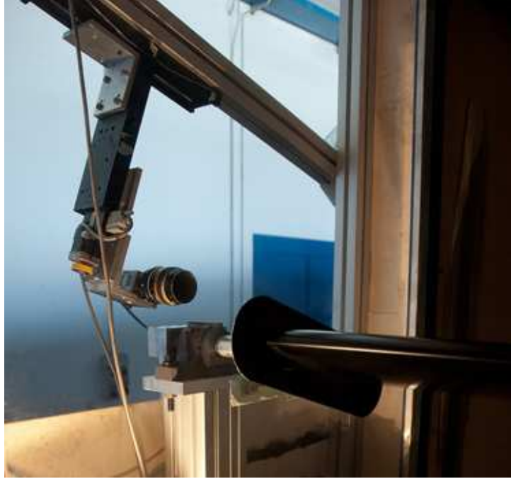
Figure 2.17: Particular of the double shutter camera mounted on a dual axis traversing system.
