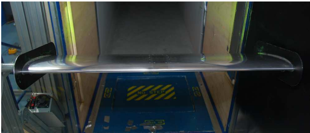
Figure 2.4: NACA 23012 blade section model inside the wind tunnel.
