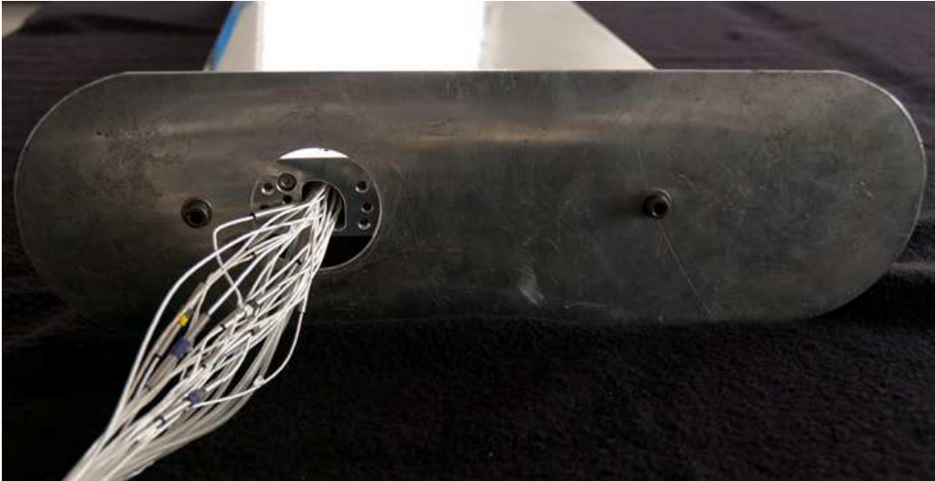
Figure 2.14: Particular of the pressure transducers cables.
