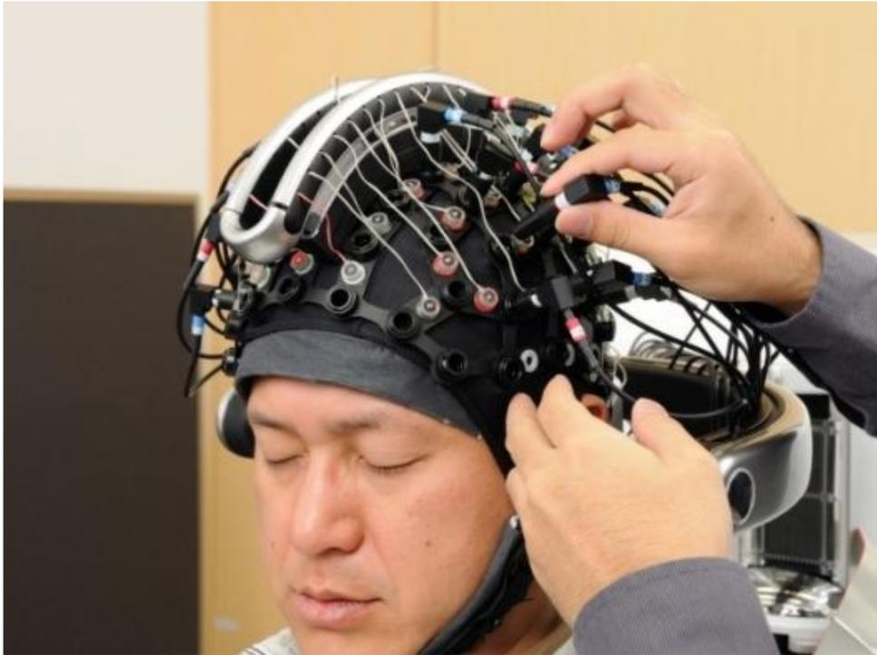
**Fig.7.1 “total brain” integrated EEG/NIRS helmet. Honda Asimo. The helmet, when connected to the NIRS and EEG devices, provides simultaneous measurement of EEG and NIRS signals from the whole brain.**
