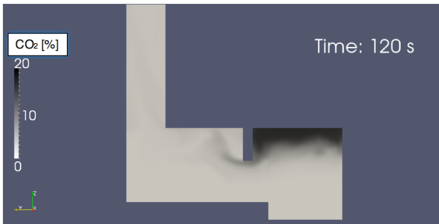
Figure 53: Smoke distribution at 120 sec nearby the exit door (represented with carbon dioxide concentration)
