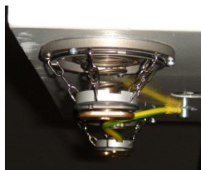
Figure 2.13. A detail of the anticollision system.
