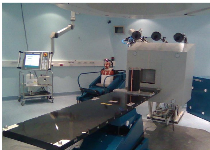
Figure 2.5. Treatment room 1. A carbon couch is docket to the PPS.
