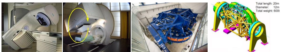
Figure 1.21. different examples of rotating gantries. From left to right: a. a linear accelerator for conventional RT; b. the proton gantry at PSI; c. the first rotating gantry for protons and carbon ions at HIT; d. a scheme of the gantry installed at HIT.
