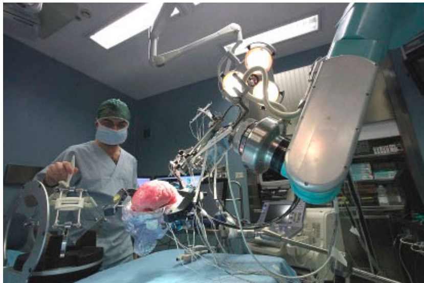
Figure 3.1: The ROBOCAST system in the operating room. The operator remotely operates an haptic interface (Omega3, Force Dimension, CH) in order to introduce straight needles inside the brain for tissue sampling or for electrode placement. The needle is driven by a rigid probe driver which is attached to a kinematic chain constituted by three robots (13 DOFs).
