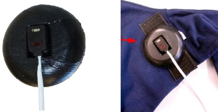
Figure 6.4: On the left the Nonin reflectance pulse oximetry sensor is inserted into the plastic holder, which, on the right, is connected to the internal side of the shoulder of the shirt.
