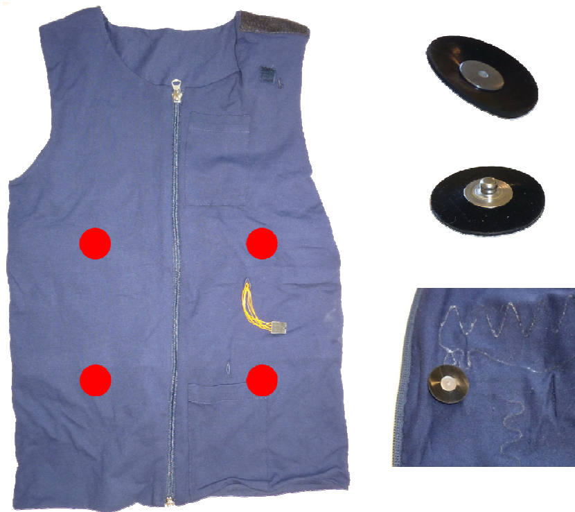
Figure 6.5: ECG electrodes shown on the upper right corner (back and forward) are connected to the shirt with snap fasteners as shown in the lower right corner. The position of the four electrodes is shown in the image on the left by the red spots.
