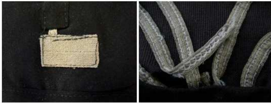
Figure 3.8: ECG electrodes. On the left the sewn silver electrode, on the right the silver bindings that bring the signal to the data handler.
