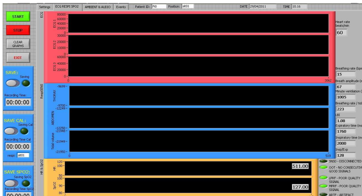
Figure 3.4: Labview® software interface for the acquisition of data transmitted by the data handler via Bluetooth for testing purposes.
