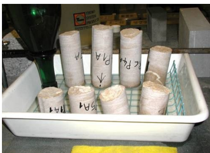
Figure 3.35: Determination of the water absorption by capillarity rise. Samples in the water and example of diagram showing the average coefficient of suction (courtesy of Arch. C. Tedeschi).
