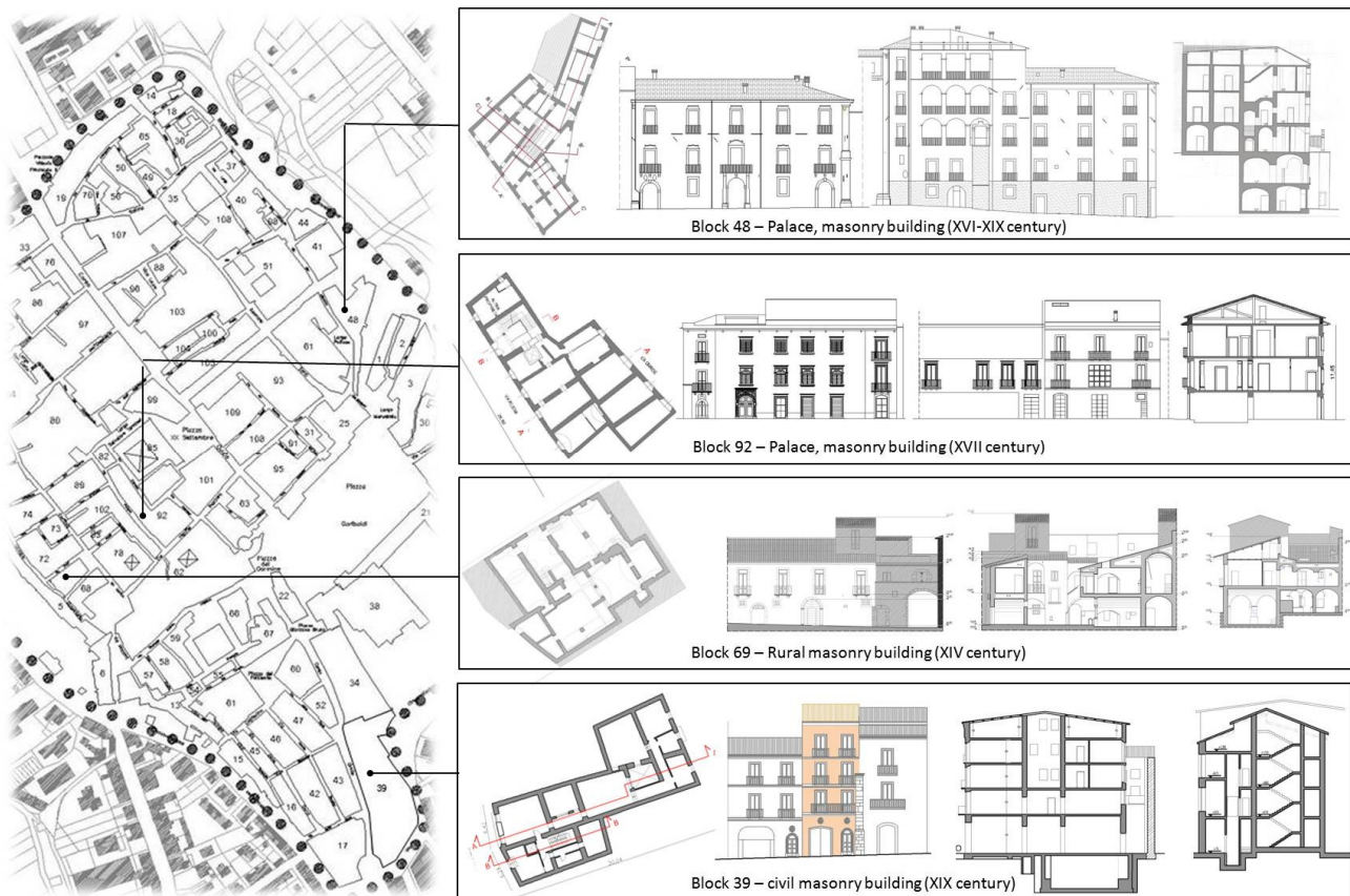
Figure 5.34: Comparison between the 4 investigated building typologies (layouts, rearranged by the author, are a courtesy of Professor A. Anzani and Arch. G. Cardani).
