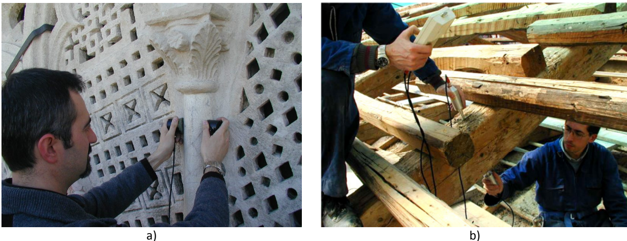
Figure 3.12: Two different transducers and receivers used for direct ultrasonic tests: a) flat devices and b) devices with wedges (pictures by the author).
