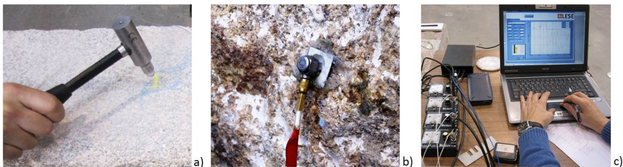
Figure 4.30: Devices used for sonic tests: a) instrumented hammer; b) accelerometer; c) computer (author's pictures).
