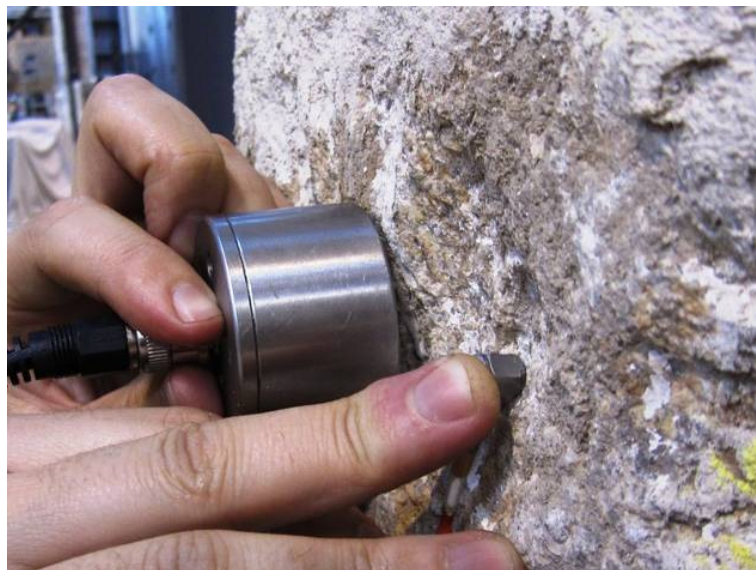
Figure 4.34: Example of bad contact between the receivers and the rough surface of a stone
