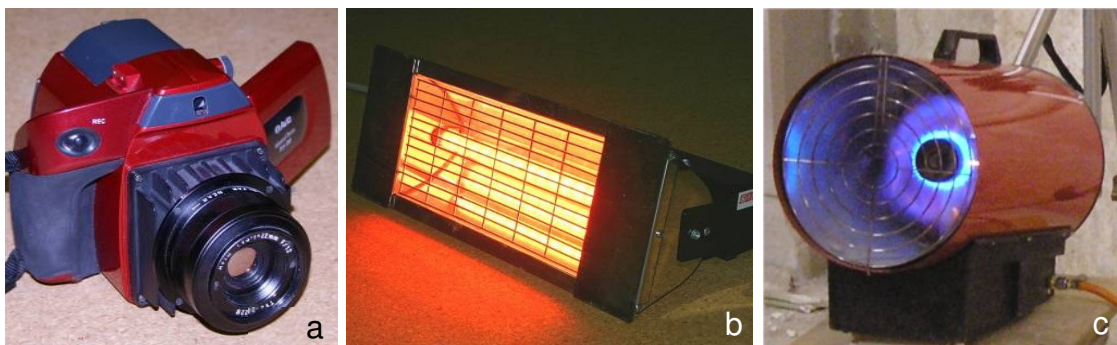
Figure 4.1: Devices used for the thermographic test: a) IR camera; b) IR lamp; c) warm air generator
