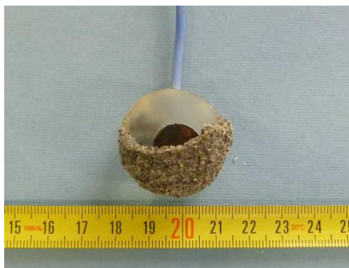
Figure 5.4 - Carbon steel specimen before pickling after 4 months AC interference (batch D)
