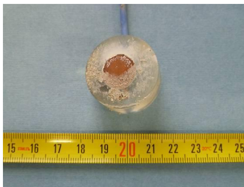
Figure 5.1 – Carbon steel specimen before pickling after 1 month AC interference (batch A)
