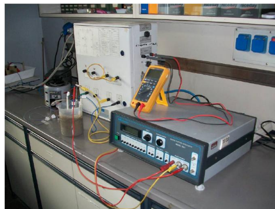
Figure 2.4 – Galvanostatic and potentiostatic tests: experimental arrangement
