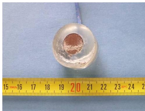
Figure 5.2 - Carbon steel specimen before pickling after 2 months AC interference (batch B)
