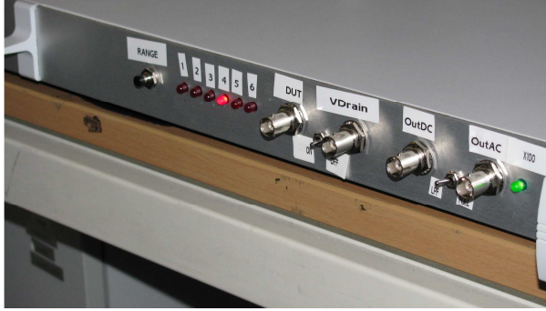
Figure 2.19: Photo of the multistage system, mounted on a rack. The terminal are easy accessible by bnc cable.
