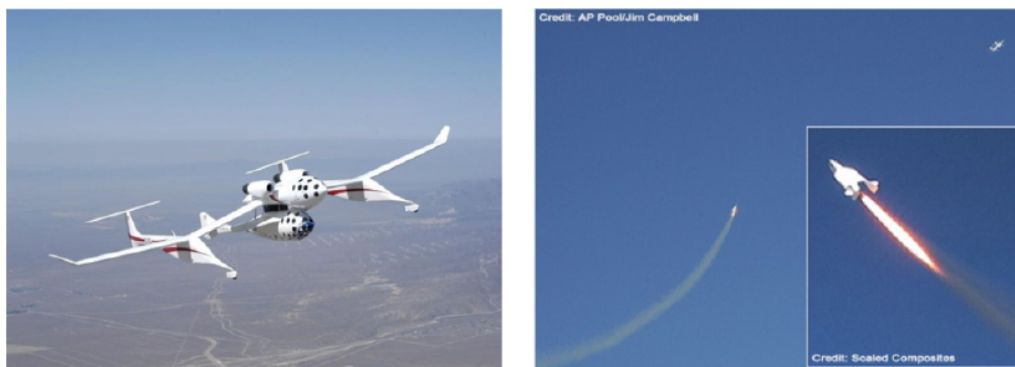
Figure 2.5: SpaceShipOne carried by the mother-aircraft White Knight (left) and during the boost phase after separation (right) [10].
