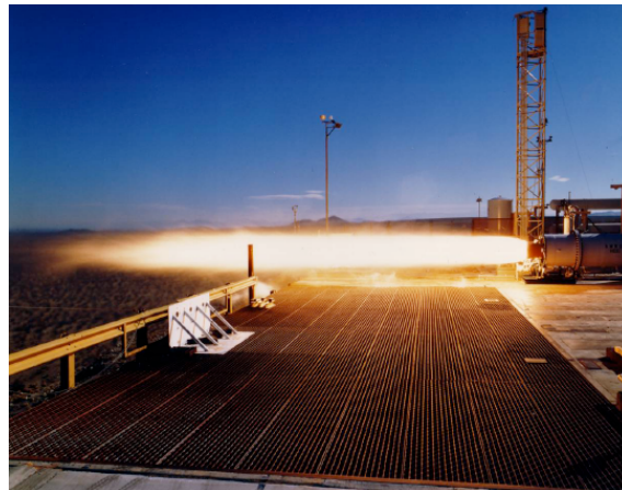
Figure 2.4: Test of AMROC H-500 motor, using LOX/HTPB as propellant [4].
