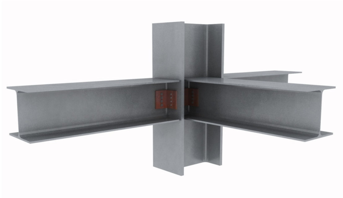
Figure 4.38 Connection of beam with column
