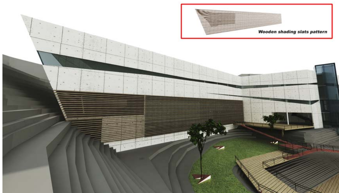
Figure 3.24 Wooden slab façade of health club
