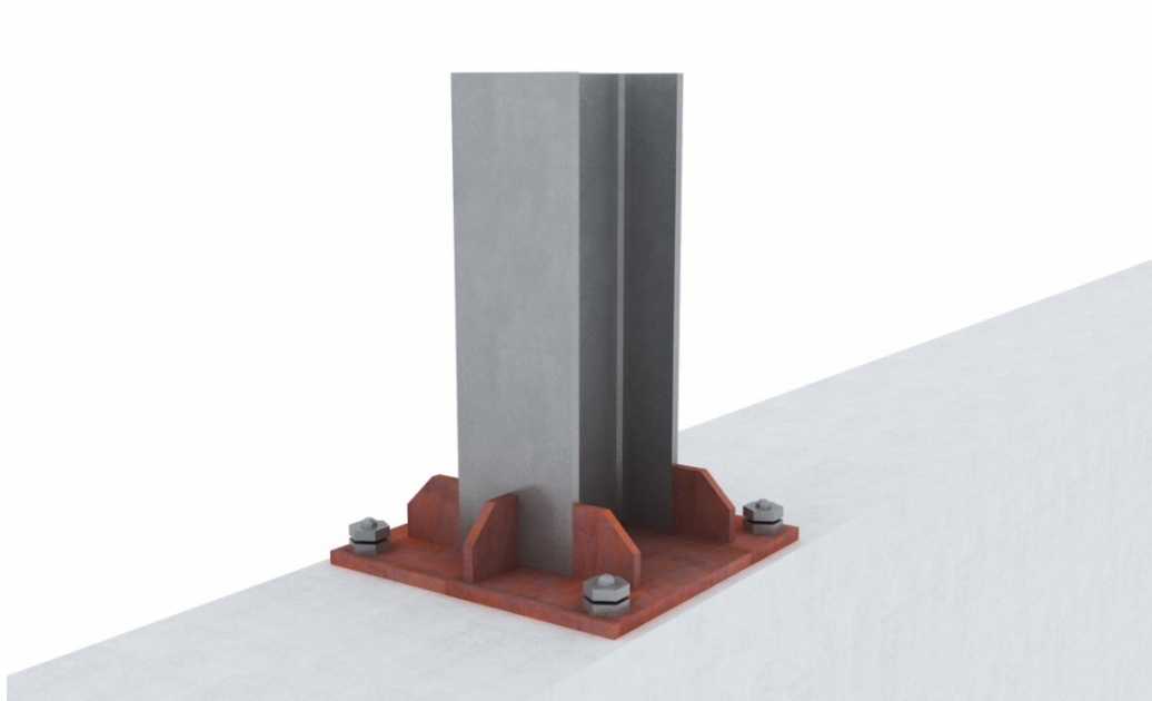
Figure 4.40 Connection of column with foundation
