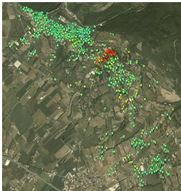
Figure 2.2: Visualization of permanent scatterer position in a example map. In red those points located in the Ivancich landslide body.
