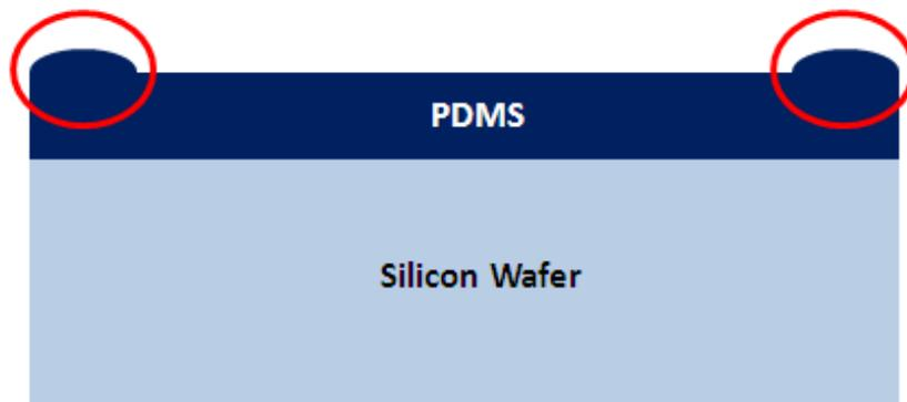
*Figure 5.1 : Locations of edge bead formed during the spin-coating of PDMS on top of the wafer*
