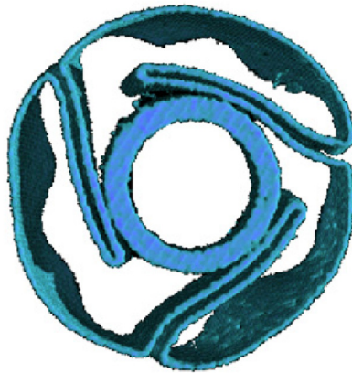
Figure 1.14 – Micro-CT based reconstruction of the trifolged balloon, coupled with the cylindrical inner shaft [25].
