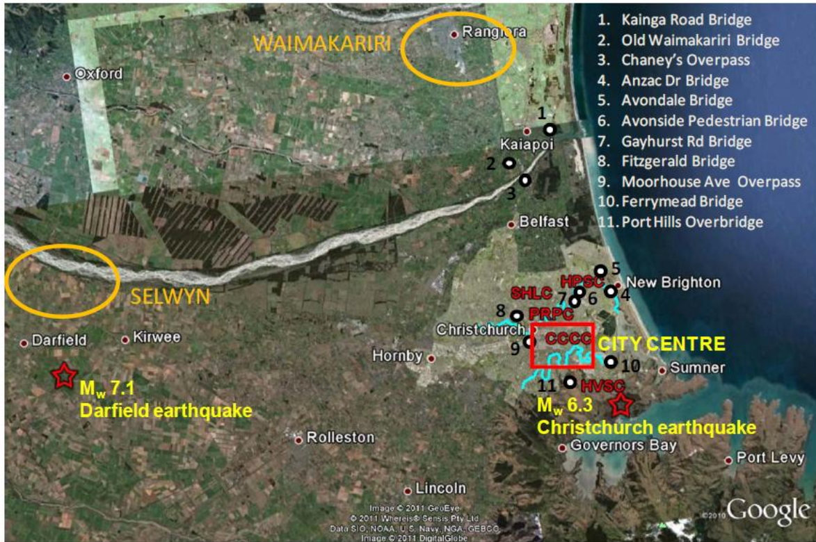
Figure 2.1. Overview of Christchurch and the surrounding region, indicating locations of a selection of damaged bridges, strong motion stations and the epicenters of the major earthquakes (Google Inc. 2011).
