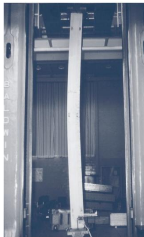
Figure 69. Example of a Buckled Column [1]
