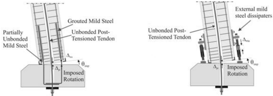
Figure 45 . Internal versus External Replaceable Dissipaters at the base of the wall [2]
