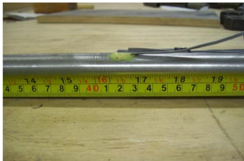
Figure 89. Strain Gauging of the Dissipator at the mid length (top), Detail of the Strain Gauging (bottom)
