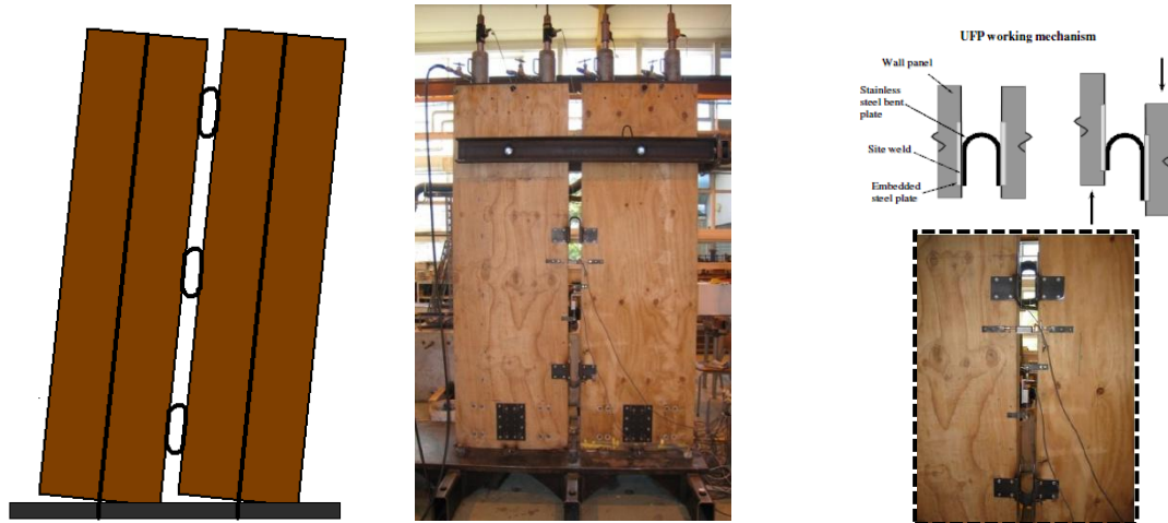
Figure 48. Scheme of Coupled Wall System with UFP devices (left), Test set up of Coupled Wall System (center), Particular of UFP devices (right) [22]
