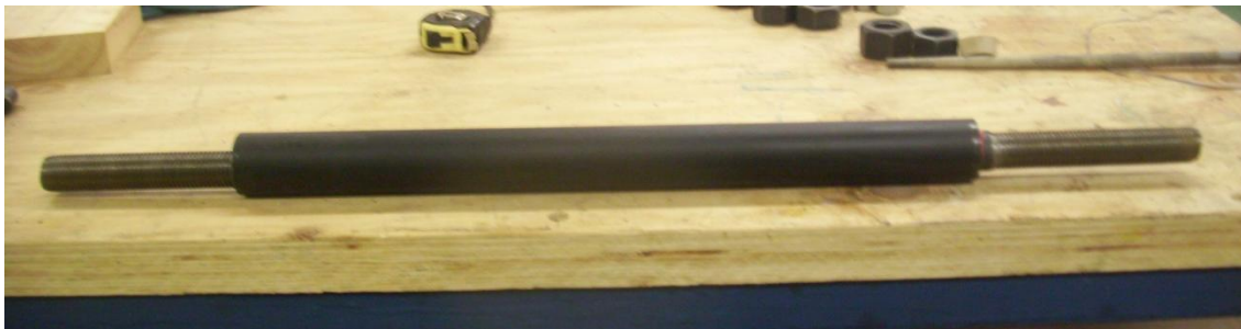
Figure 51. Example of Plug and Play dissipator: Schemratic Design (top), Example of a Dissipator (bottom)
