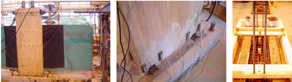
Figure 46. (a) Hybrid Timber Wall with Internal Dissipaters, (b) Energy Dissipation Devices, (c) Wall base [1]
