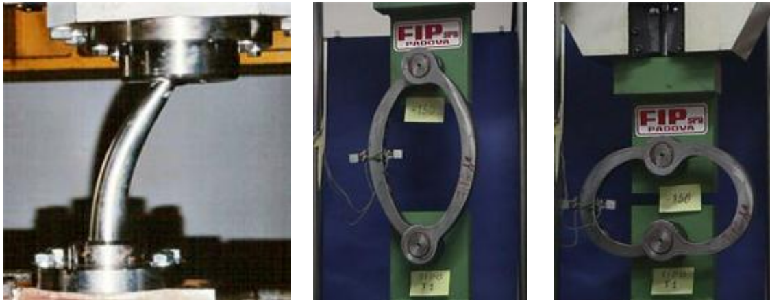
Figure 12. Pin shaped damper (left); Crescent moon shaped damper; Butterfly shaped damper
