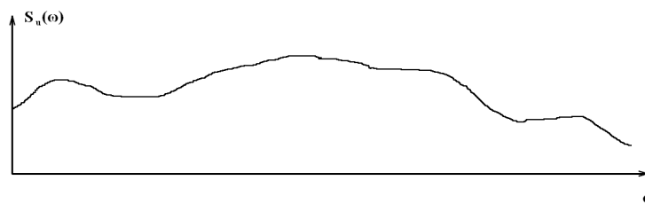
Figure A- 8 Power spectral density function of a sinusoidal signal with disturb
