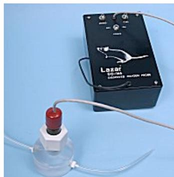
**Figura 6.1** Sensori Micro Flow Through  $O_2$  and  $pO_2$  Electrodes (Lazar Research Laboratories, Inc., CA, USA) e relativa centralina di controllo.
