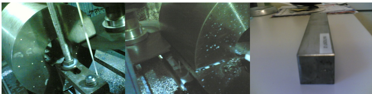
Figure 3.3.3 Cutting process of the specimen.
