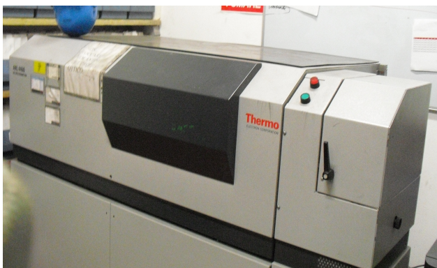
Figure 2.5.8 - Quantometer used for the determination of metallic aluminium content in the ingots.
