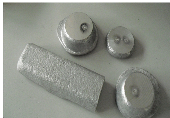
Figure 2.5.9 - Metal ingots after OES analysis.
