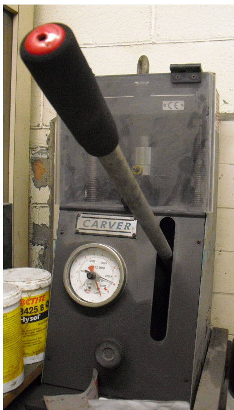
Figure 2.5.6 - Press machine used for the preparation of the tablets.
