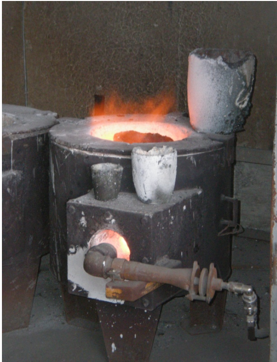
G) The residual material above 0.8 mm (coarse fraction) was melted in a crucible in order to recover the non-ferrous metal content [9].
