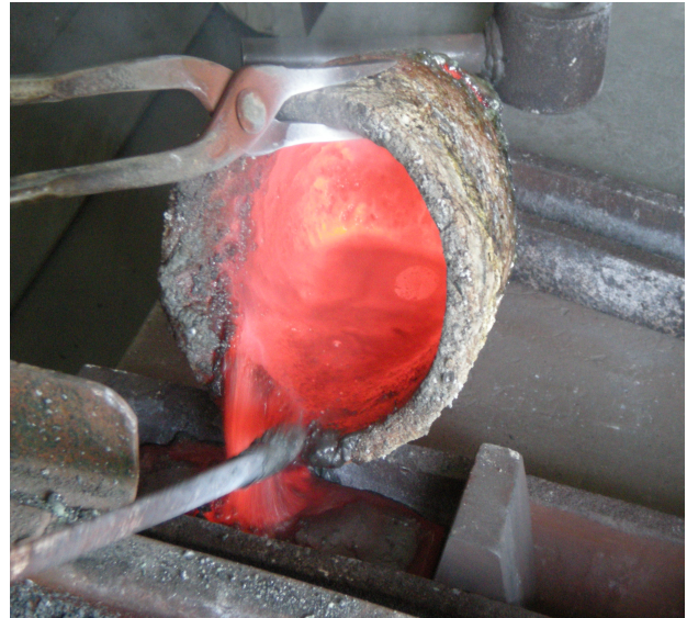
H) Detail of the casting process: aluminium metal and other non-ferrous metals aggregate into droplets that float above the surface of the molten salts. Therefore, they are easily separated through a casting process that results in the formation of a metal ingot. The remaining salt dross is casted separately in a mould where it cools down and it is conserved for further analysis.
