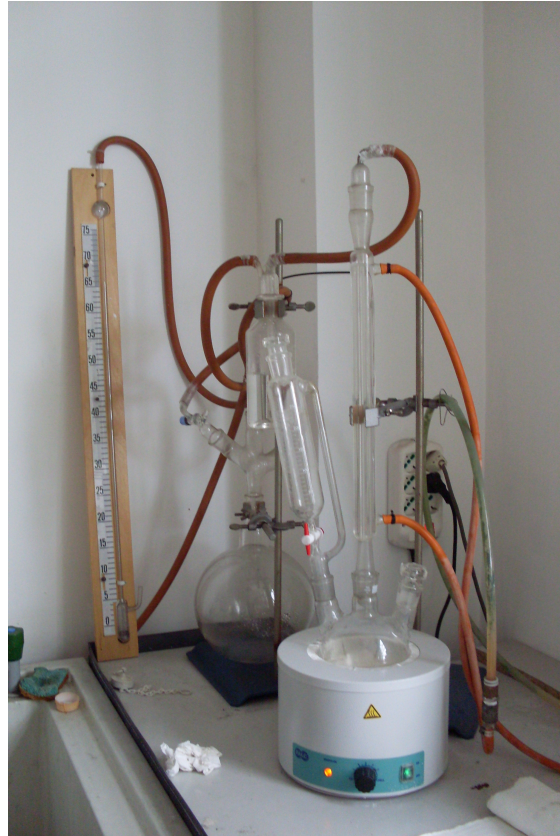
Figure 2.5.3 - Laboratory device used to measure metallic aluminium content with the “soda attack” method.
