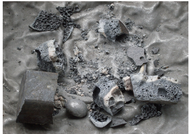
L) The salt dross resulting from the melting process was first grinded and then screened at 0.8 mm. The fraction below 0.8 mm was analyzed with the same procedure as for bottom ash fine fractions. In the dross of several samples it was possible to find aluminium droplets lost during the melting process.
