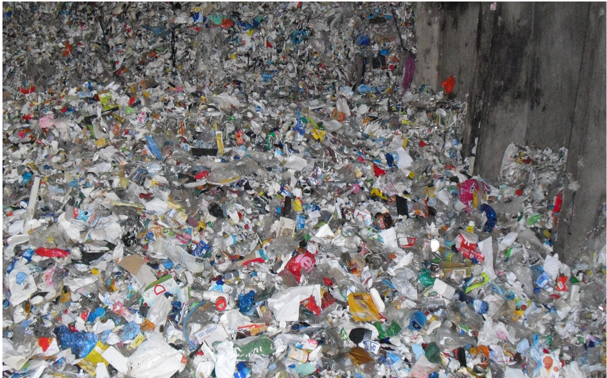
Figure 2.3.2 - Doped waste charge preparation: residual waste from Seruso plant (mainly plastic and paper).
