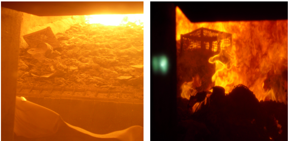
Figure 2.3.6 - Cages in the furnace right before the discharge in the quenching water.
