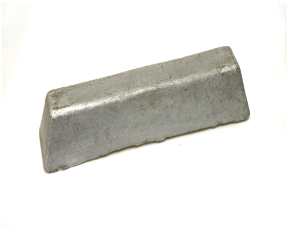
I) The metal ingot resulting from the melting process was weighted and sent to OES analysis in order to assess its aluminium content.
