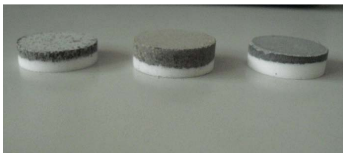
Figure 2.5.5 - Sample tablets ready for XRF analysis.
