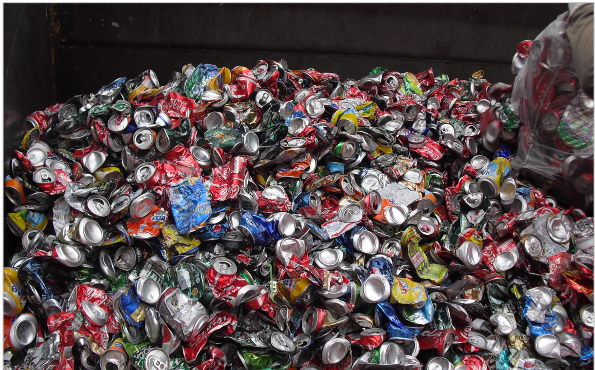
Figure 2.3.3 - Doped waste charge preparation: aluminium beverage cans used for Test 1 (6 th of June 2011).
