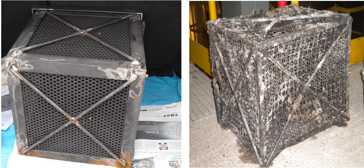
Figure 2.3.5 - Cage before and after the test.
