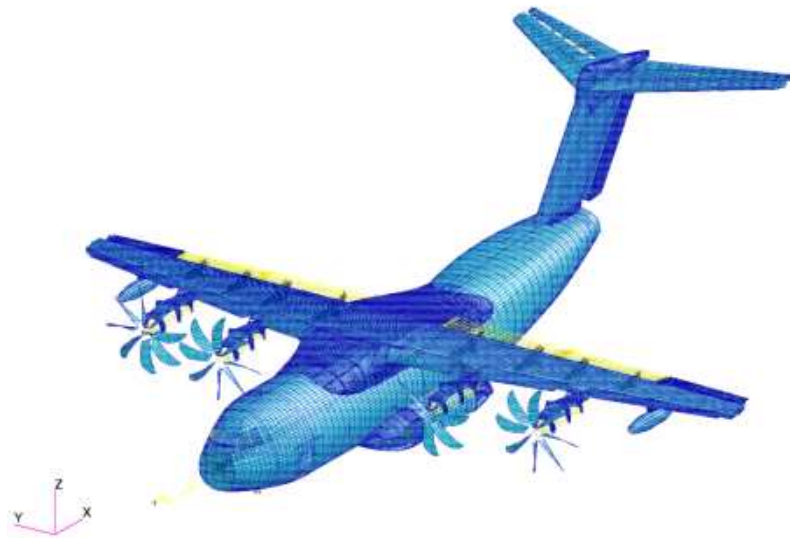
Figure 4.2. A400M FE model.
