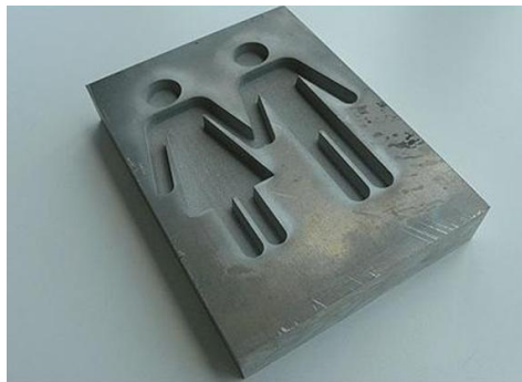
Figure 2.14.: An example of abrasive water jet milling, that uses the same nozzle and garnet abrasive that is used for conventional water jet metal cutting.
