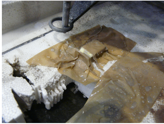
Figure 7.5.: The fixturing system is composed by polystyrene and sellotape
