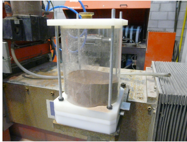
Figure 6.2.: The self-made mini hopper installed in the water jet system.
