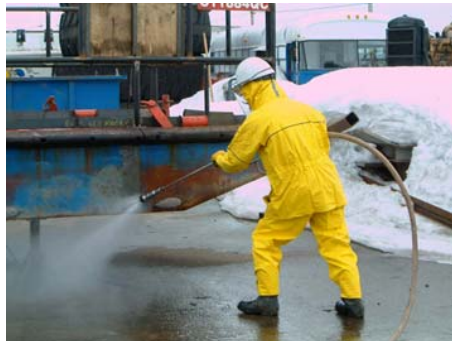
Figure 2.16.: Water jet polishing: sea and salt removal
