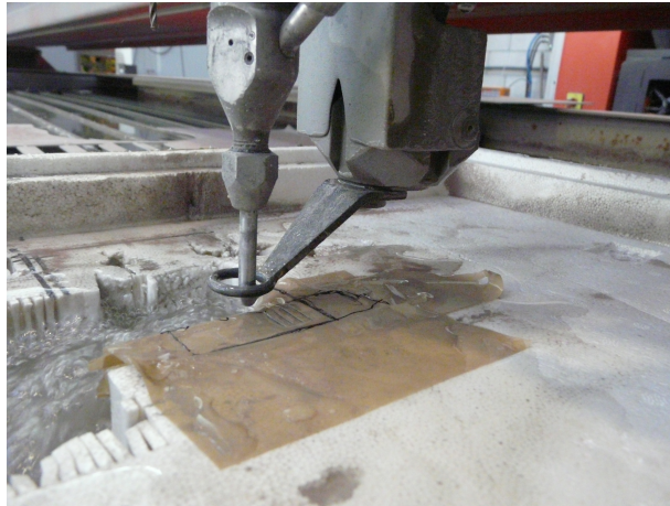
Figure 6.9.: The fixturing system used during this experimentation.
