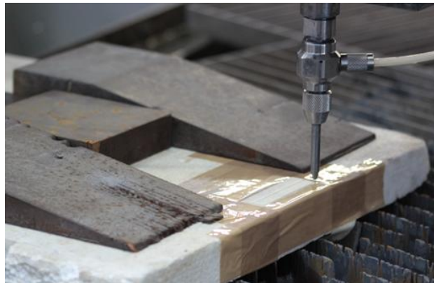
Figure 5.10.: The fixturing system used during the feasibility experiments.
