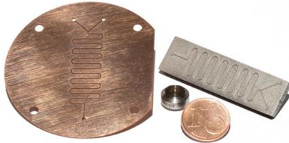
Figure 3.5.: Copper electrode sheet machined by WJ, 80 \mu\text{m} WJ nozzle and the final tool produced by MEDM.
