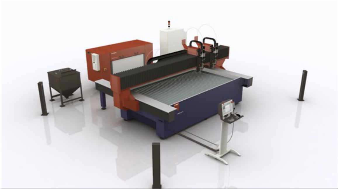
Figure C.1.: Water jet cutting system used in this experimentation
