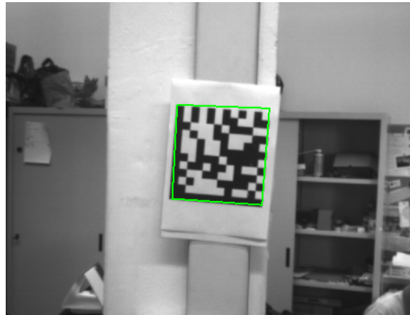
Figure 4.10: Data Matrix detection with libdmtx corners
