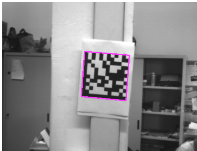
Figure 4.15: Data Matrix final contour with GFTT
