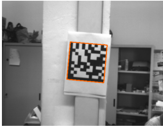
Figure 4.20: Data Matrix final contour with Canny
