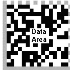
Figure 3.5: ECC 200 Data Matrix encoded data
