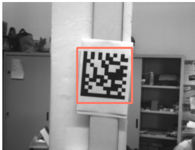
Figure 4.11: Region-Of-Interest inside which compute GFTT algorithm
