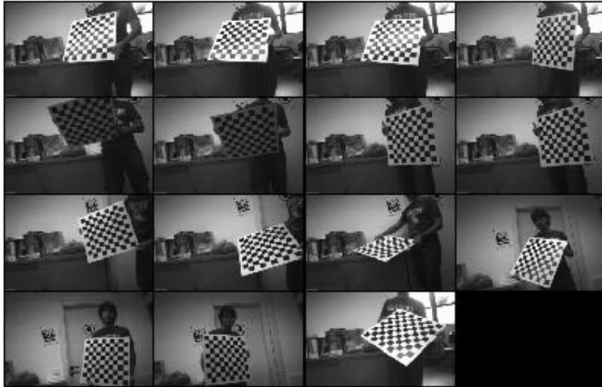
Figure 4.3: Chessboard images for camera calibration
