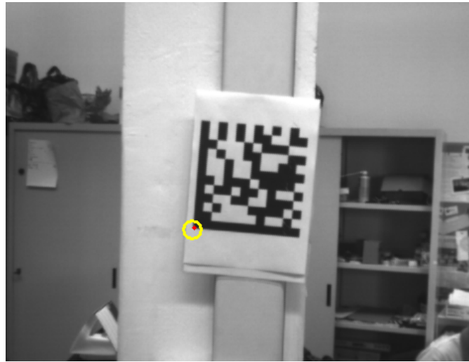
Figure 4.12: GFTT mask for bottom-left point detection
