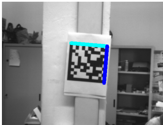
Figure 4.13: Linear masks for top and right edges in the first sweep
