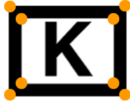
Figure 2.1: Fiducial Marker with alphabet 'K' and detected corners.
