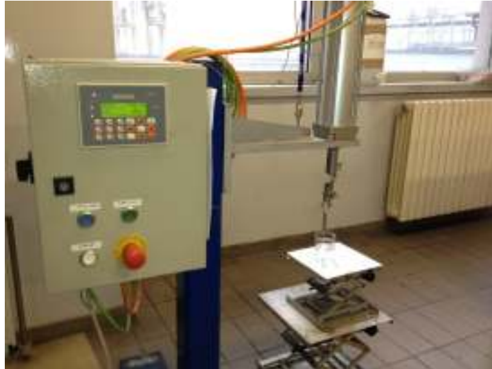
Figure 2.1 Dip coating of the titanium grade 2 samples
