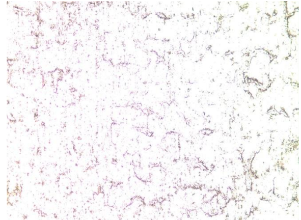
Microscopic image 100x (Aluminum, No Pretreatment, No Paint). Before Potentiodynamic test.
