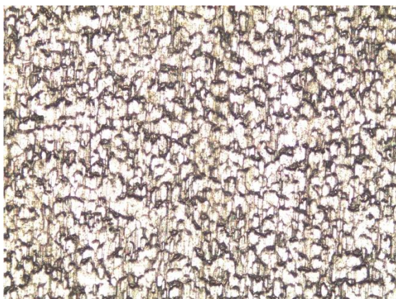
Microscopic image 50x (Aluminum, ZnPh, No Paint). Before Potentiodynamic test.
