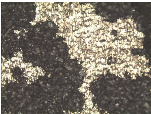
Microscopic image 50x (Aluminum, No Pretreatment, No Paint). After Potentiodynamic test Without Nitrogen.
